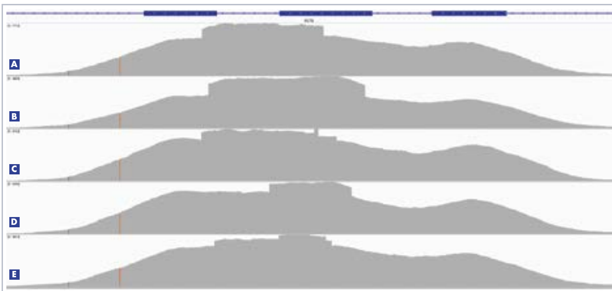
Figure 2: Facilitated by OGT's expert bait design, FLT3 -ITDs of various sizes and even regions containing multiple ITDs can be confidently detected. ITD sizes are A 174 bp, B 225 bp, C 195 bp with additional 6 bp, D 120 bp and E 168 bp with additional 69 bp.
